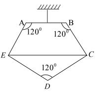
reaction at the joint D is of magnitude  $b\sqrt{3}w$  and find the thrust in the light rod CE.
